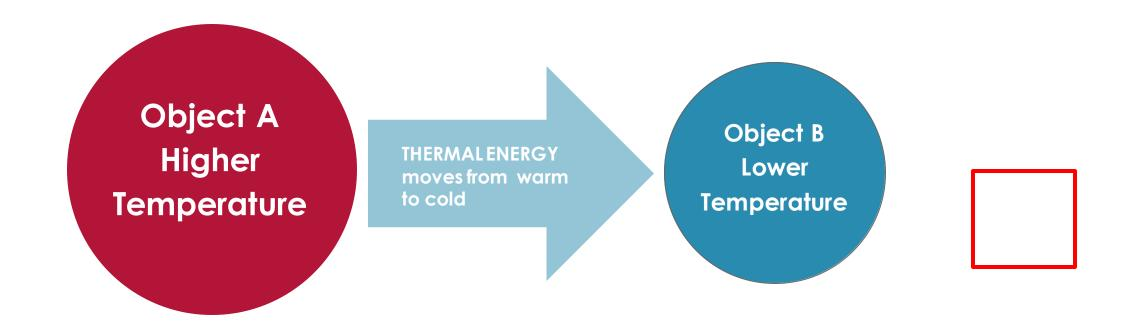
Thermal Energy always flows from the object or material with a higher temperature towards the object or material with a lower temperature (the Second Law of Thermodynamics).
