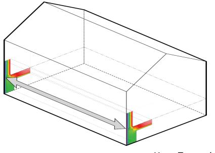
The heat loss coefficient of a linear thermal bridge is the loss of energy associated with that thermal bridge (W/K)
